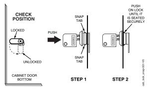
Figure 1. Installing the Cabinet Lock
